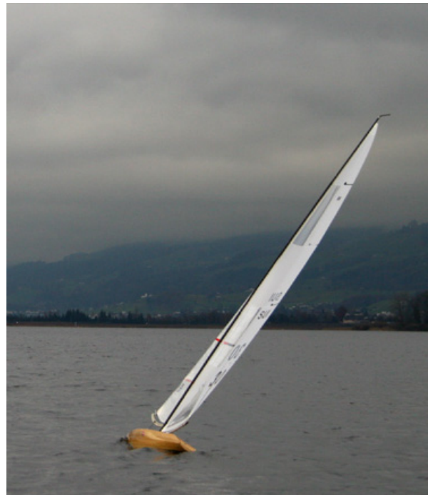
FIGURE 4 Remote-controlled 2 m tall model boat featuring a front sail constructed with laminated Vectra® foils produced in this work (Chapter IV), illustrating a possible application, which could be up-scaled in the future. The weight saving of the sail was determined to be 30 %, while its performance is highly improved in terms of strength and stiffness.
