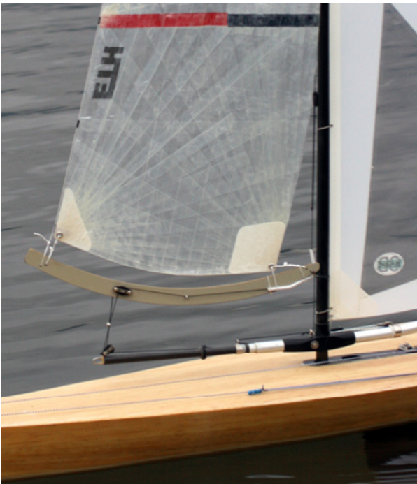
FIGURE 4 Remote-controlled 2 m tall model boat featuring a front sail constructed with laminated Vectra® foils produced in this work (Chapter IV), illustrating a possible application, which could be up-scaled in the future. The weight saving of the sail was determined to be 30 %, while its performance is highly improved in terms of strength and stiffness.
