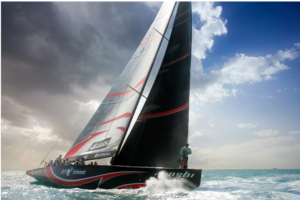
FIGURE 8 2007 America's Cup Defender Team Alinghi testing their new experimental front sail (genoa), constructed with Createx Amalgame spread-fiber technology. 64 The mainsail is a North Sails Group 3DL ® product. 62 Photograph reprinted with permission. 65
