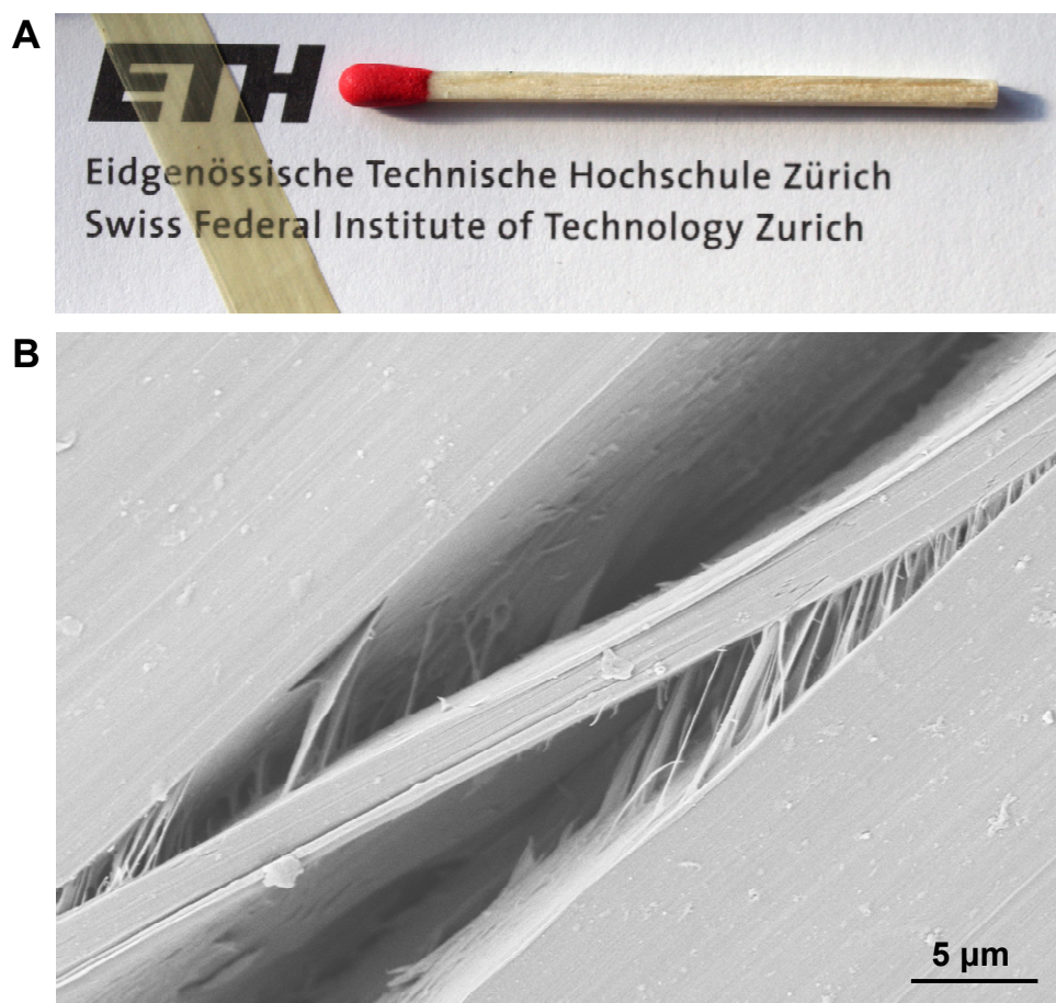
FIGURE 2 A. Optical photograph of a dried PPTA foil placed on top of letter head, illustrating its transparency. The width of the foil is 8 mm. B. Scanning electron micrograph of an as-extruded, dried foil that was spliced longitudinally.
